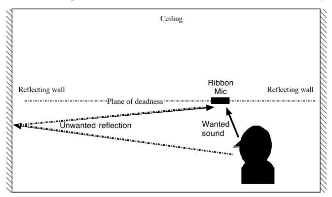
HORIZONTALLY-MOUNTED RIBBON MIC REJECTING WALL REFLECTIONS
